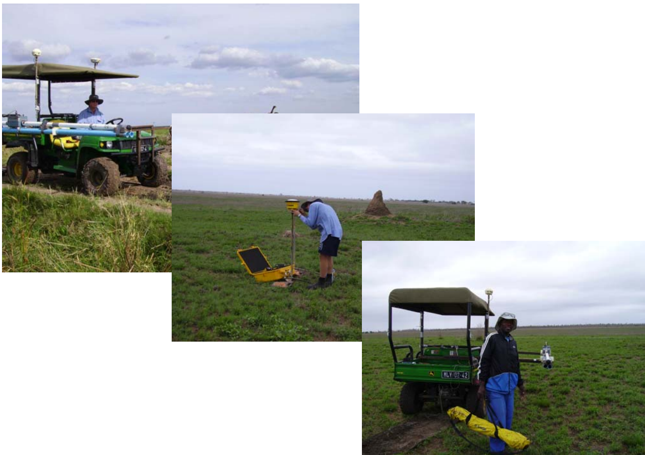
Fig.4 : Electromagnetic induction instruments and RTK GPS mounted on a four wheeled bike
