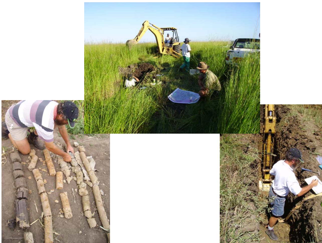
Fig.6 : Detailed soil investigations conducted at locations based on the apparent conductivity maps
