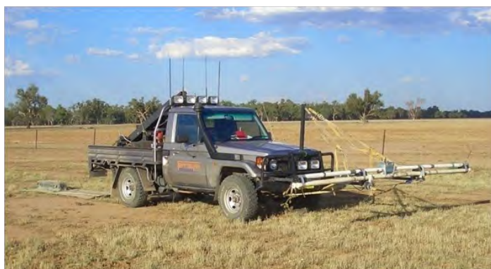
EM31/38 soil survey rig can be mounted on a 4WD or quad bike.
